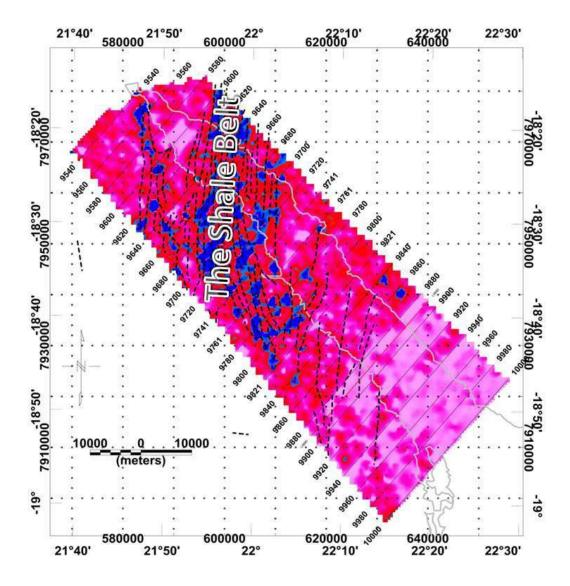
The Shale Belt in northwestern Botswana as delineated from airborne electromagnetic data. The background image is the resistivity distribution at a depth slice of 400m (red tones are resistive areas whereas blue zones show conductive areas). Drilling results have shown that the conductors are carbonaceous shales/metapelites, hence The Shale Belt. Broken lines are magnetic basement grain mapped from aeromag (notice the good correlation between the magnetic structure and the conductors)
