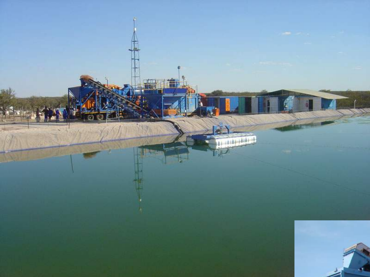
10 tph DMS bulk sampling plant purchased and installed in Letlhakane.
