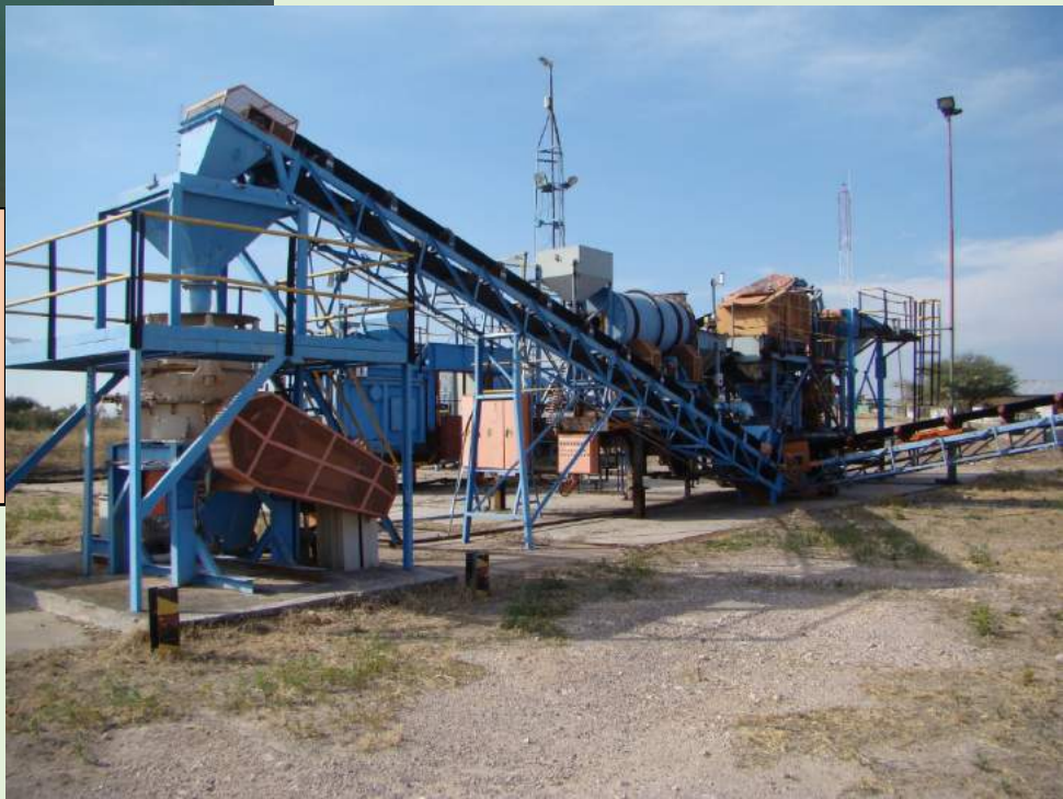
10 tph DMS bulk sampling plant purchased and installed in Letlhakane.
