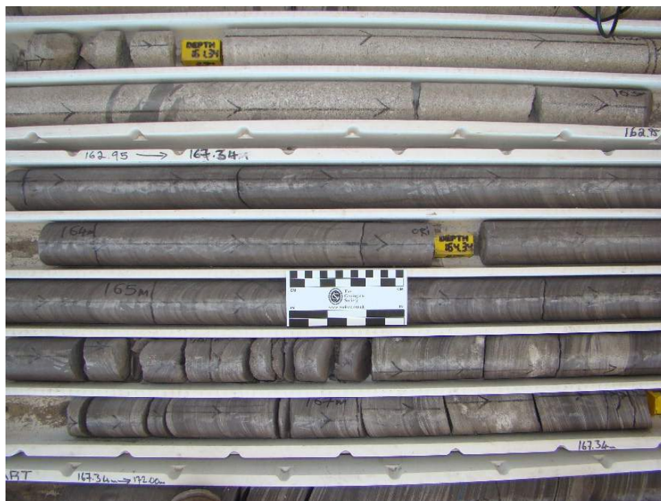
Figure 7. Borehole BWADD0014. Section 162 to 168 meters has high values of radioactivity which are mainly carbonaceous siltstones.
